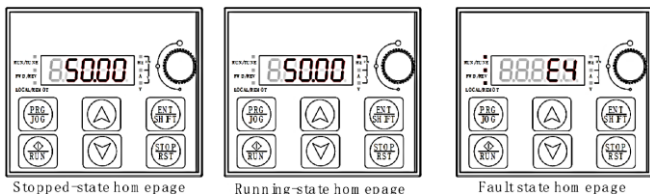
Figure 5-2 Status interface display
